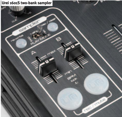
loop playing until released - much like a cue button on a CD player. The 25mm volume sliders for each bank also work as triggers in 1-shot mode when they are pushed up from the off position, but unlike the trigger pads, the loop will keep playing. This is great for working out when you want the loop to start, say on an off beat for example.
