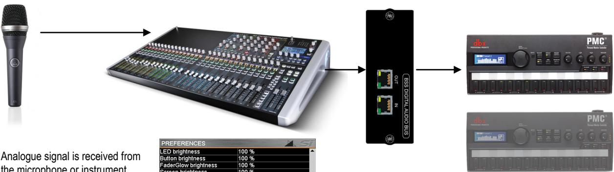
Analogue signal is received from the microphone or instrument and the engineer applies the optimum amount of gain to avoid input overload.
