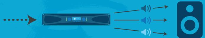
These speakers contain a passive crossover, which splits the frequency band of the audio signal and sends each band directly to the loud speaker, requiring an outside amplifier to pass audio.
