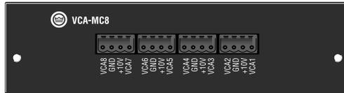
Four-pin removable Phoenix-style barrier connectors provide the +10 VDC control voltage, ground, and control inputs for two amplifier channels. Thus, the 4-channel CTs 4200 uses two connectors; the 8-channel CTs 8200 uses four connectors. The control inputs are labeled VCA1 (for channel 1), VCA2 (for channel 2), and so on.
