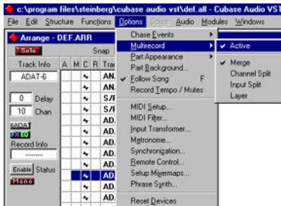
Multi-Record selection is required to record multiple channels of audio simultaneously. Please note, this selection also allows multiple MIDI streams to be recorded at the same time, the other items in this menu refer only to MIDI.
