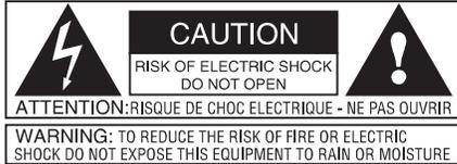
The symbols shown above are internationally accepted symbols that warn of potential hazards with electrical products. The lightning flash with arrowpoint in an equilateral triangle means that there are dangerous voltages present within the unit. The exclamation point in an equilateral triangle indicates that it is necessary for the user to refer to the owner's manual.
